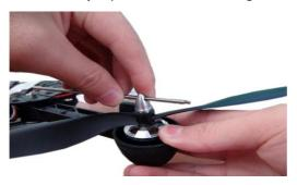
3rd step: screw up propeller clamp with screw driver.
