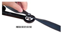
> 2nd step: put motor shaft through the hole of propeller clamp
